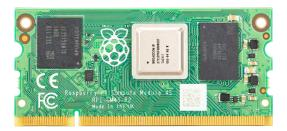
Raspberry Pi Compute Module 4 SODIMM (CM4S) is a System on Module (SoM) containing processor, memory, eMMC flash, and supporting power circuitry. These modules allow a designer to leverage the Raspberry Pi hardware and software stack in their own custom systems and form factors. The SODIMM form factor compute modules have 18 additional GPIO pins compared to the standard Raspberry Pi boards, for a total of 46, opening up more options for designers.
